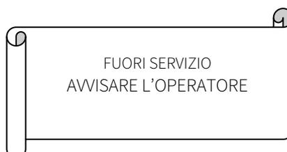
This message means that the program is corrupt and the change machine board must be reprogrammed.
