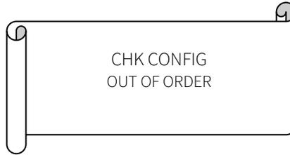
This message means that the configuration and accounting data of the change machine are corrupt and it is therefore necessary to set accounting to zero and to reconfigure the board.
